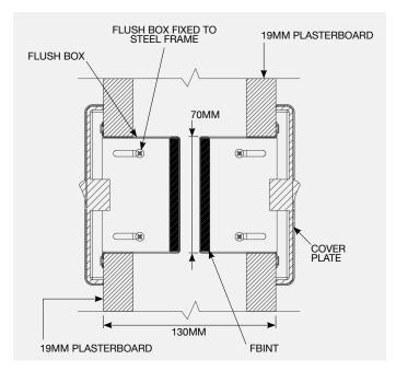
**Detail 1** is a back to back installation on a hollow wall system comprised of a 92mm steel frame and 1 x layer of 19mm Fireline on each side of the frame (total wall thickness of 130mm). The FBINT was installed into a standard flush mount galvanised steel box, measuring approximately 75mm high x 50mm wide x 52mm deep.
