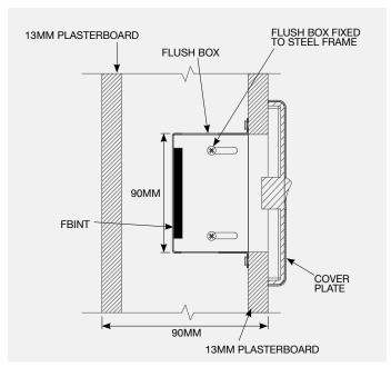
**Detail 2** is a one side test on a 13mm plasterboard, 64mm frame and 13mm plasterboard setup (total wall thickness of 90mm). The FBINT was installed into a universal galvanised steel flush box, measuring approximately 90mm high x 50mm wide x 52mm deep.
